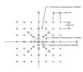
3/8-16 THREADED MOUNTING HOLES IN CENTER AND CIRCULAR PATTERNS
